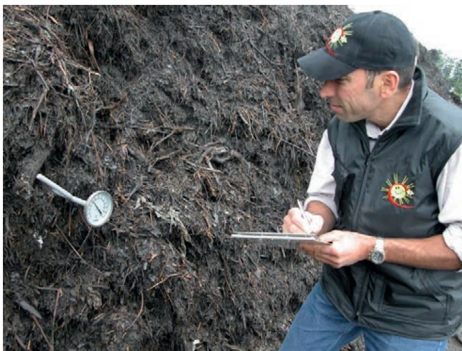
Figure 4.3 Temperature measurement is important to control the composting process.
